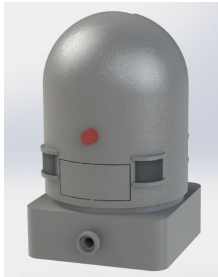
Figure A.3.1.1 Flud’s user interface from the hardware perspective, including the power button, hose opening, and battery casing
