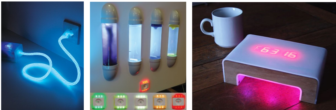
Figure 2-9. Ambient energy displays (left to right): (a) Power-Aware Cord (b) Watt-I-See ambient energy source visualization (top) and power draw visualization (bottom) (c) Wattson Energy Monitor
