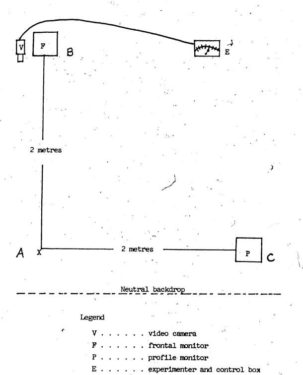
Figure 1. Schematic layout of the video camera apparatus for assessing body size perception.
