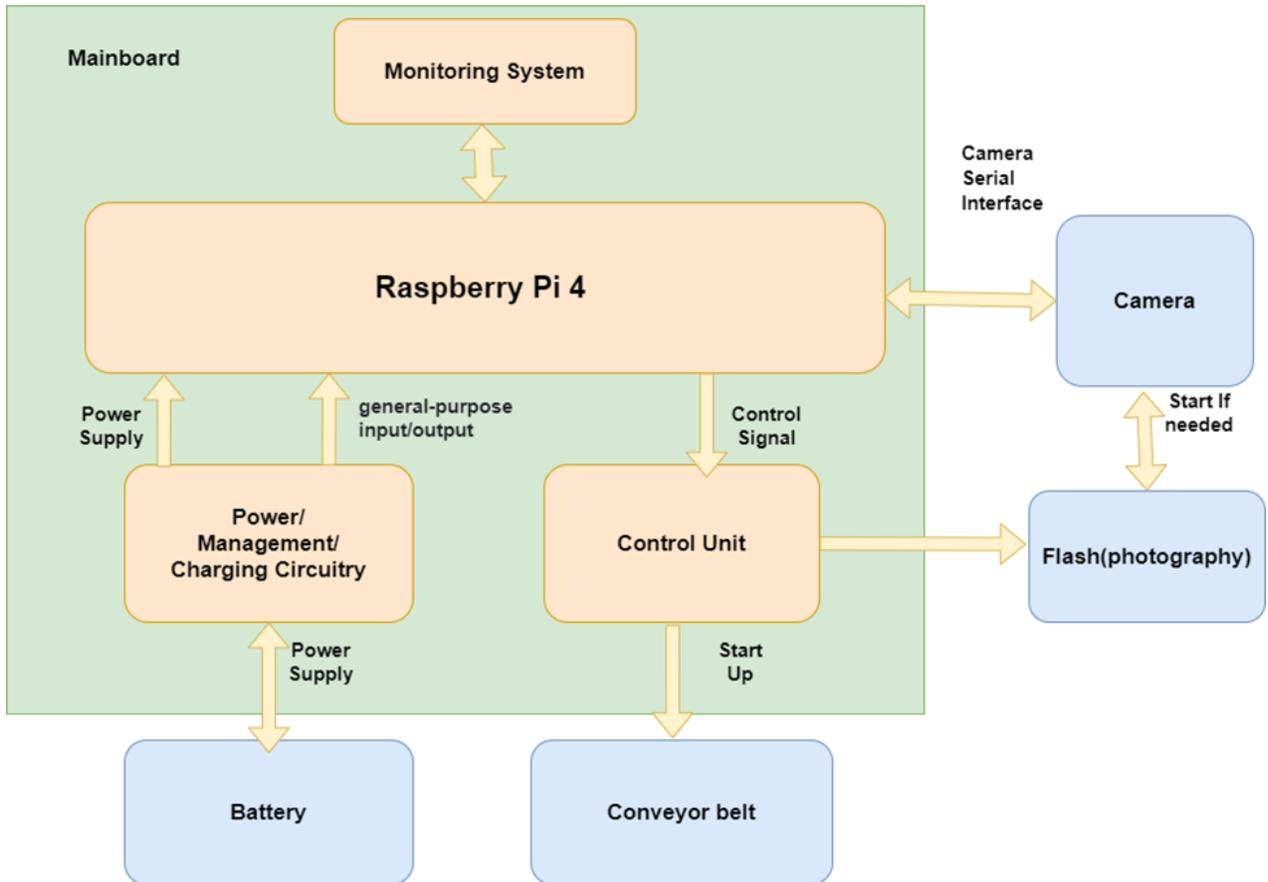
Figure 2.4 - Sort-e System Block Diagram
