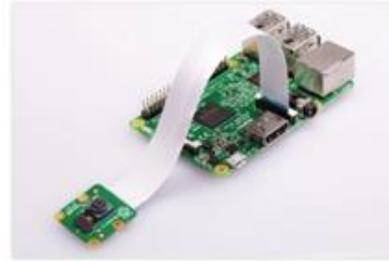
Figure 2.3: Camera Module V2 [12]
