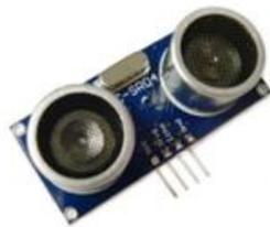
Figure 2.5: HC-SR04 Ultrasonic Sensors [14]
