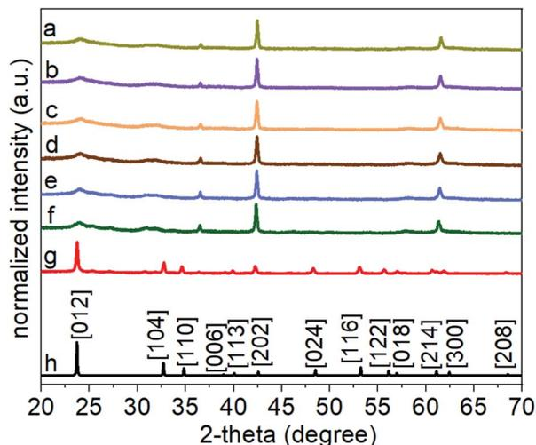
Fig. 2 The X-ray diffraction (XRD) patterns for the  $\text{LiNbO}_3$  product, obtained after a 24 h hydrothermal process, following its heat treatment to: (a) 30 °C; (b) 100 °C; (c) 200 °C; (d) 300 °C; (e) 400 °C; (f) 500 °C; and (g) 600 °C. (h) A reported  $\text{LiNbO}_3$  reference (ICSD No. 28294) is included for comparison. The diffraction patterns were each normalized by dividing their intensities by the maximum diffraction intensity within each pattern.
