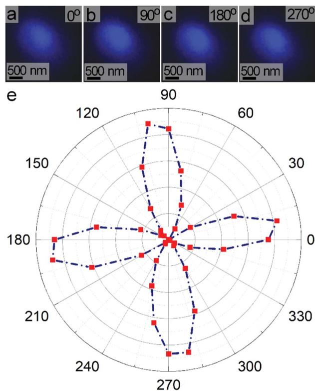
Fig. 8 Images of the SHG response of a single, mesoporous LiNbO<sub>3</sub> particle as a function of polarization of the excitation at distinct angles: (a) 0°; (b) 90°; (c) 180°; and (d) 270°. (e) A polar plot of the SHG response (in arbitrary units) generated using an excitation wavelength of 800 nm for a single LiNbO<sub>3</sub> particle. This plot shows the dependence of the resulting intensity of the SH on the polarization of the excitation beam.
