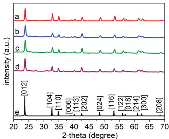
Fig. 3 Powder X-ray diffraction (XRD) patterns of calcined  $\text{LiNbO}_3$  particles, which were originally prepared by hydrothermal reaction times of: (a) 24 h; (b) 48 h; (c) 72 h; and (d) 96 h. Also included are XRD patterns for (e) a reported  $\text{LiNbO}_3$  reference (ICSD No. 28294).
