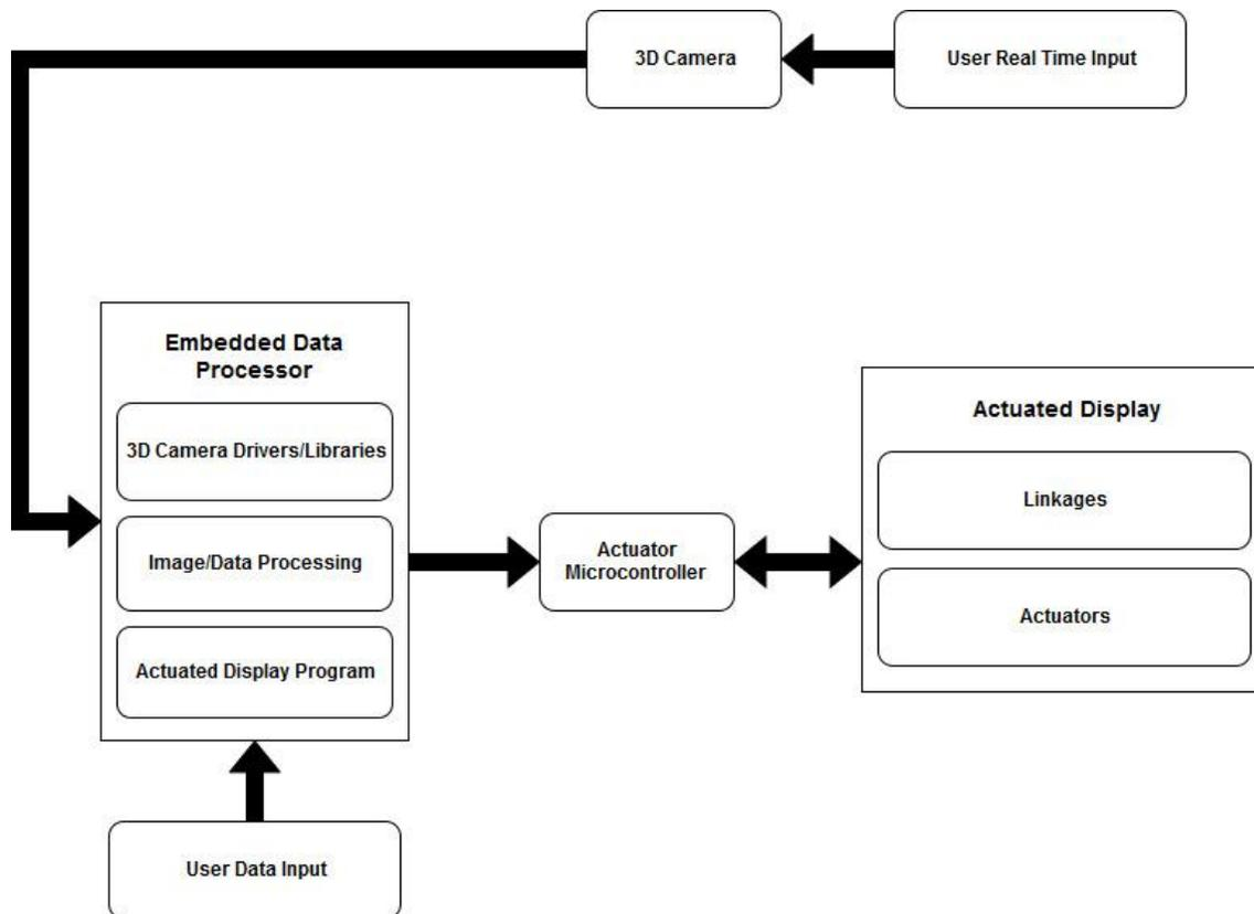
Figure 2: High-level functional block diagram of *Relevo*
