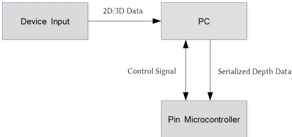
Figure 4: Software system block diagram of *Relevo*
