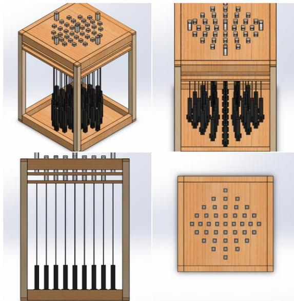
Figure 3: CAD simulated view of *Relevo*
