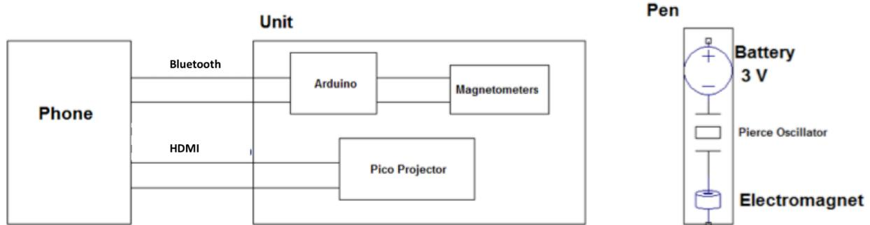
Figure 5- Hardware Systems Diagram
