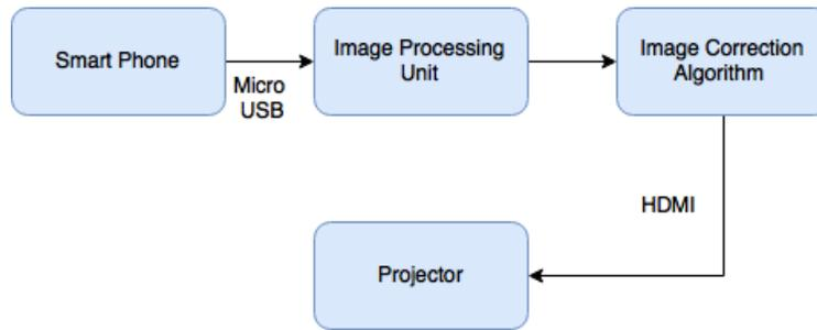
Figure 3- Conceptual Diagram of the Projection Unit
