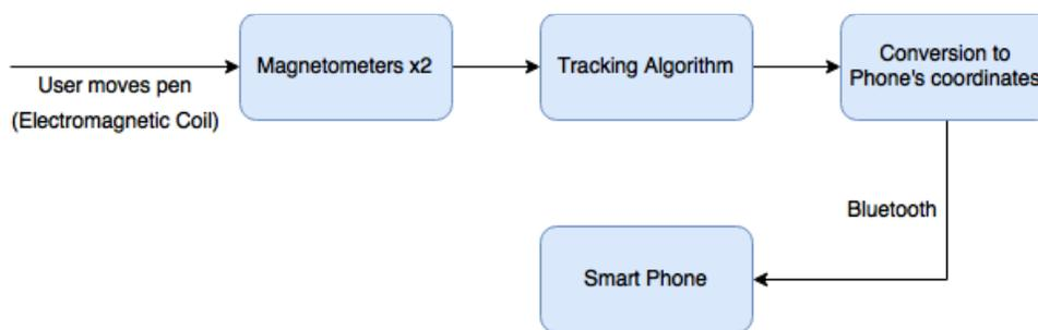
Figure 4- Conceptual Diagram of the Pen Tracking Unit
