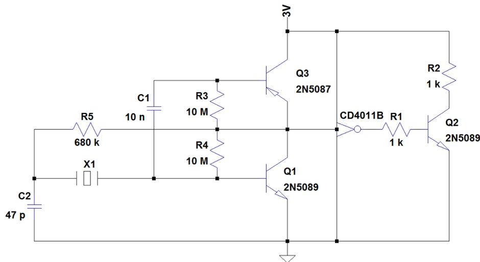
Figure 6-Pierce Oscillator Resonator
