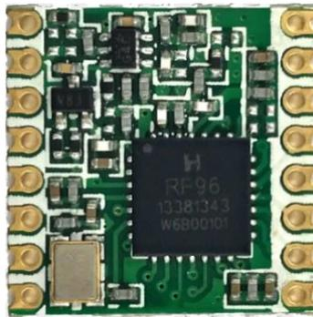
Figure 2.3: RFM96/98W RF transceiver V1.0 [2]
