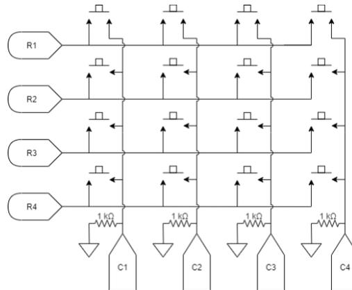
Figure 3.3.5: 4x4 button matrix schematic
