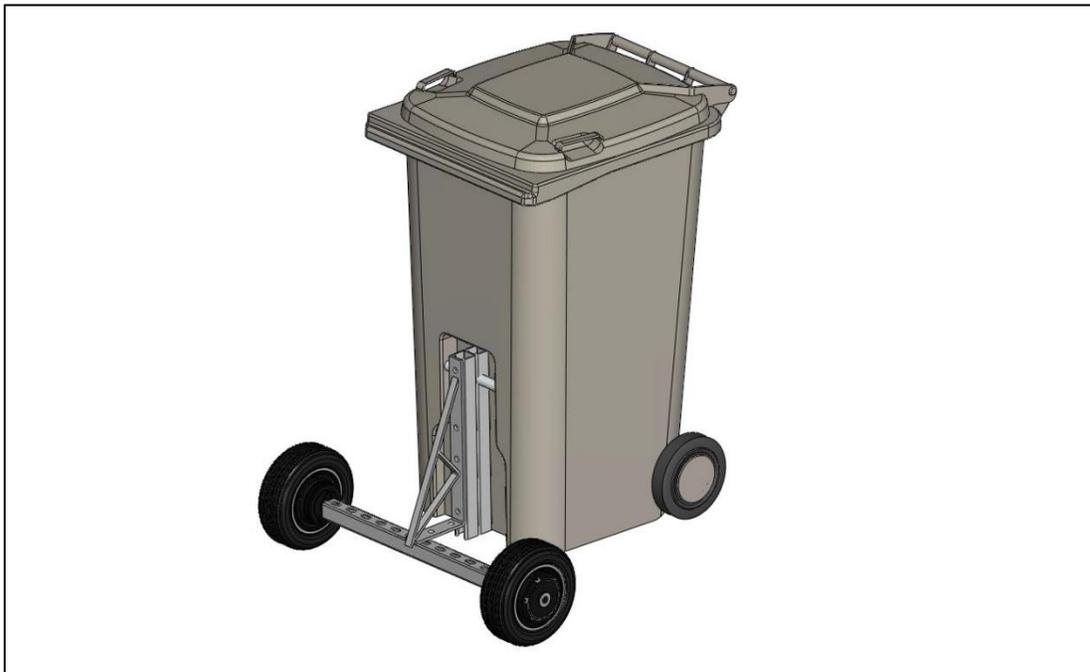
**Figure 2. 1: Conceptual Design of the Bin Buddy Attached to a 210 L Waste Cart**
