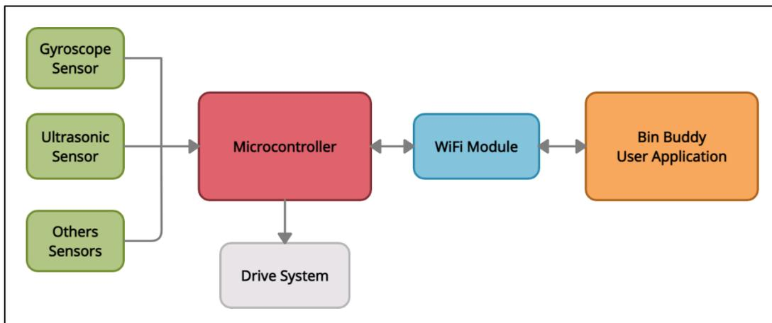
**Figure 2.2: General System Diagram**
