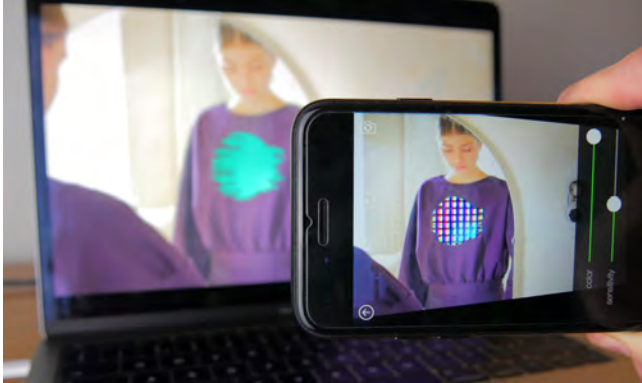
Figure 5. Activating the dynamic fabric via the chroma-key app via the computer screen
