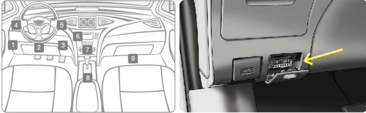
Figure 2-2: Example of a OBD-II Diagnostic Port Location
