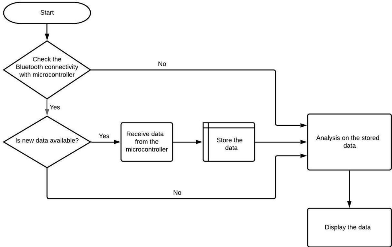
**Figure 5: Layout for Mobile Software**
