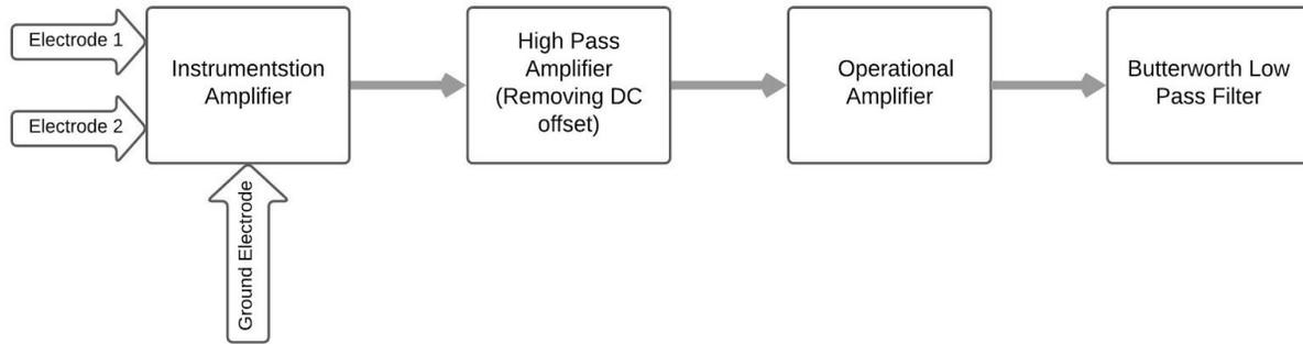
**Figure 3: Layout of Amplification Circuit**
