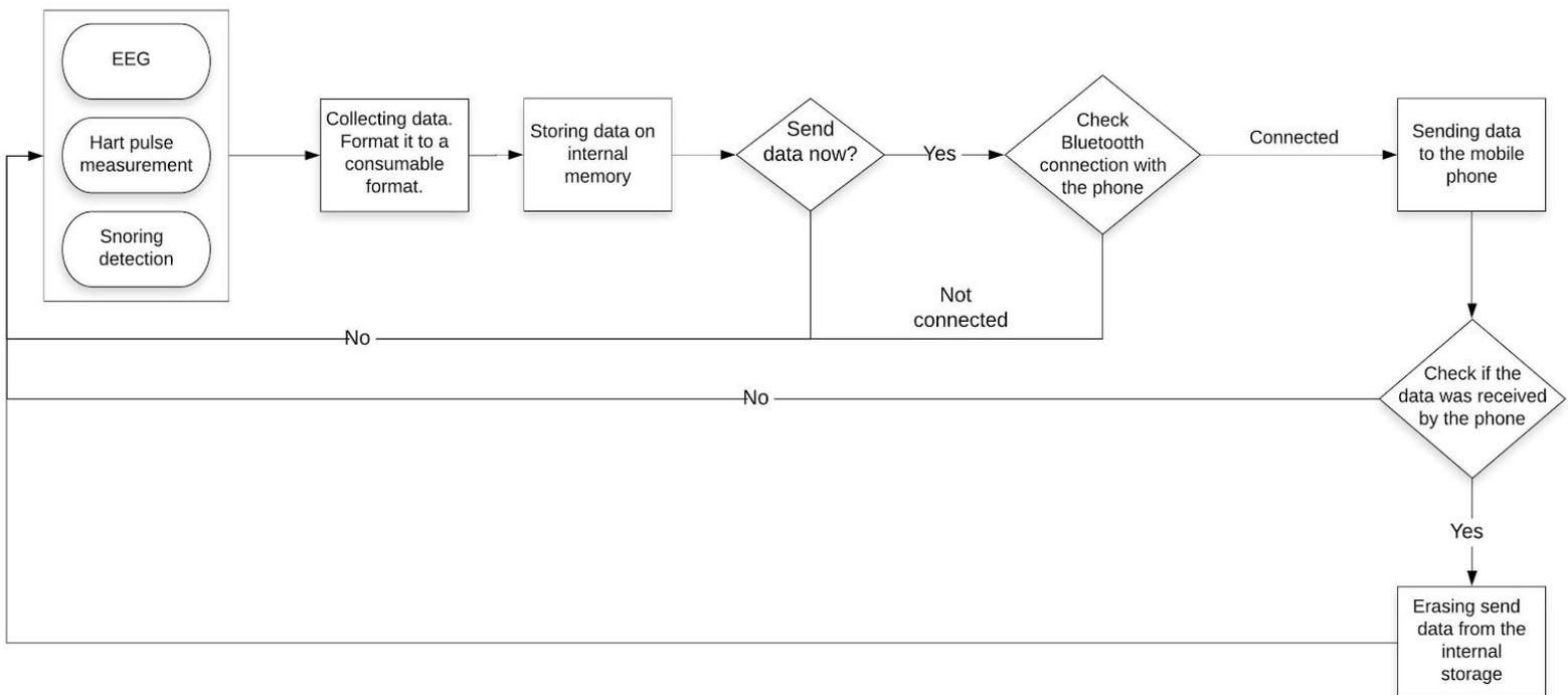
**Figure 4: Data Flow in a Microcontroller System**
