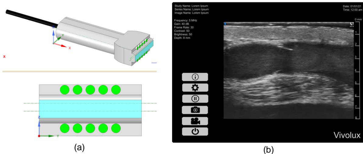
Figure 3.2.1: User interface examples (a) A 3D CAD model of the handheld probe (b) Example GUI for the general use of the device
