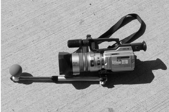
Figure 1. Camera with gray sphere attached
