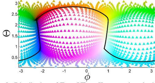
Figure 3: Distribution of Type I/Type II spectra in spherical coordinates. A regular sampling of the wavelength domain in 4nm steps was used to generate  $\lambda_1$  and  $\lambda_2$  values defining the optimal reflectance functions. Illuminant D65 and the CIE 1931 2° observer were used to calculate the sensor responses before converting to spherical coordinates. The black line indicates the boundary between Type I and Type II.
