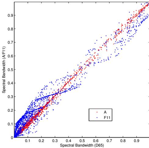
Figure 9: The illuminant-induced shifts for the 1600 glossy Munsell chips in reparametrized spectral bandwidth  $\delta$ . The significant differences in the illuminant spectrum create a larger effect for F11, which is a fluorescent light with narrow peaks in the power distribution.
