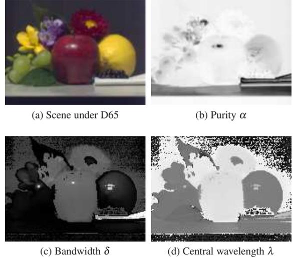
Figure 5: The  $\alpha\delta\lambda$  color descriptors calculated for a scene under D65. The original XYZ were calculated from the spectral reflectance image based on the CIE 1931 2° standard observer. The maximum angular error threshold (see Equation 3) was set to 0.05°.
