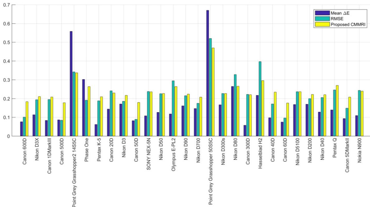
Figure 2: Plot of the three camera color accuracy measures CMMRI, RMSE (data from [2]), and mean  $\Delta E$  (data from [2]). For clarity of the comparison, the  $\Delta E$  and RMSE data are each scaled separately to match the CMMRI as closely as possible in terms of RMSE)
