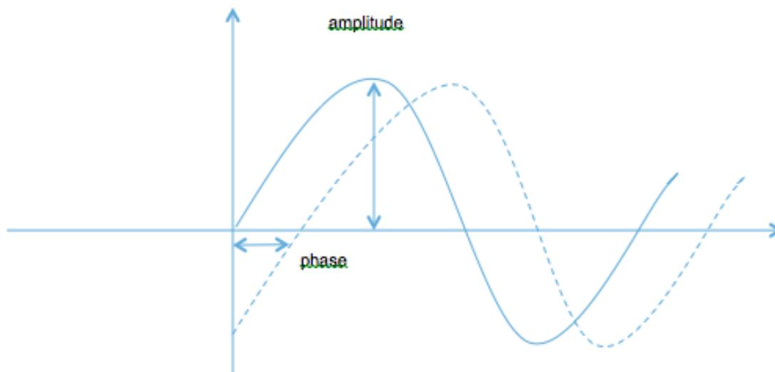
**Figure 4.5. Phase difference and amplitude of a sine wave.**
