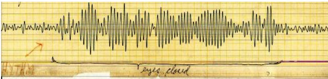
**Figure 1.1.** The first recorded MEG signal using the SQUID technology used in present day MEG systems. This signal represents the alpha rhythm, in this instance generated by opening and closing the eyes. Copyright 1972 by David Cohen. Adapted with permission.
