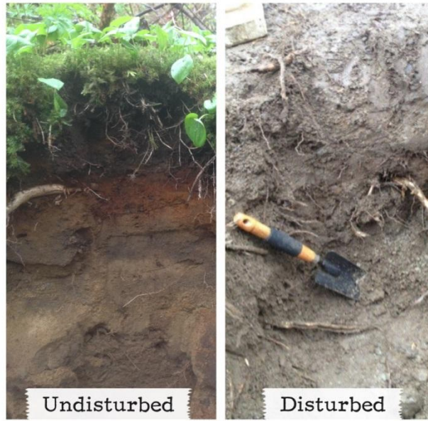
Figure 6. Comparison of disturbed and undisturbed soils. Clear layering is shown in undisturbed soil but not in the disturbed soil.
