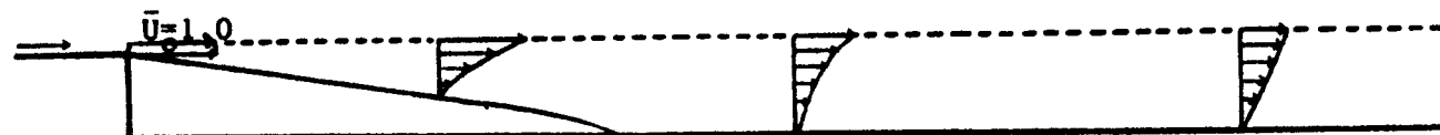
Figure 8b. Vertical velocity profile of axial jet (along center-line). Scale is 1 cm to 10 cm.
