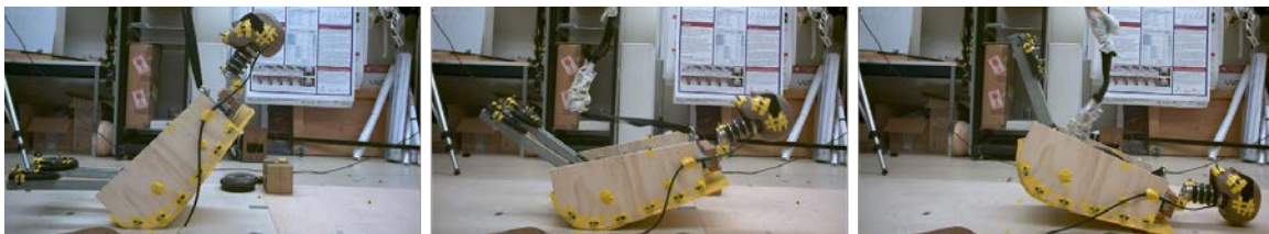
Figure 11. Sequence of images showing a sample dummy fall simulation. The figure shows the dummy in a curved torso with fixed hips configuration (CTFH) leading to head impact on a plywood impact surface.
