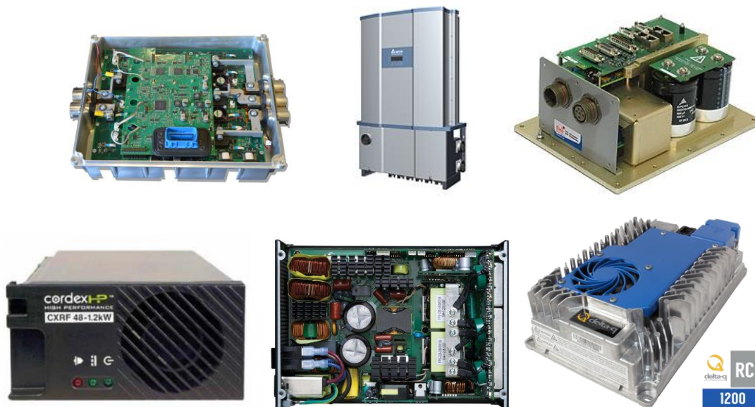
Fig. 2: Power electronics examples: Top left: Bitron Electronics’s power inverter for electric vehicles [21]; Top middle: Delta’s solar inverter [22]; Top right: Elmo’s servo drive for wind turbines [23]; Bottom left: Alpha’s rectifier for telecom [24]; Bottom middle: Corsair’s power supply for PCs [25] and Bottom right: Delta-Q’s battery charger for utility vehicles [26].
