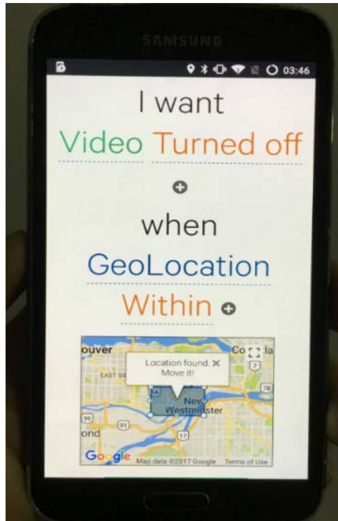
Figure 2.2 The rule-based interface of Streamer.Space, the toolkit for creating context-aware mobile video streaming apps
