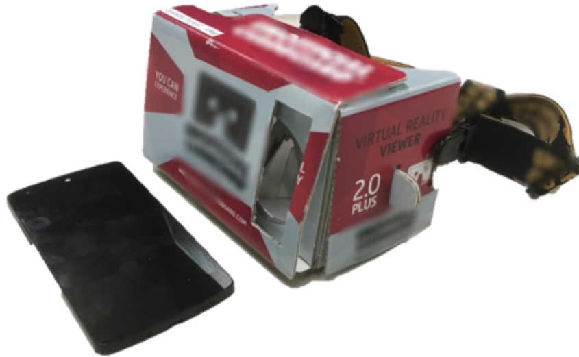
Figure 1.2 My FPV system is made with cardboard goggle and smartphone
