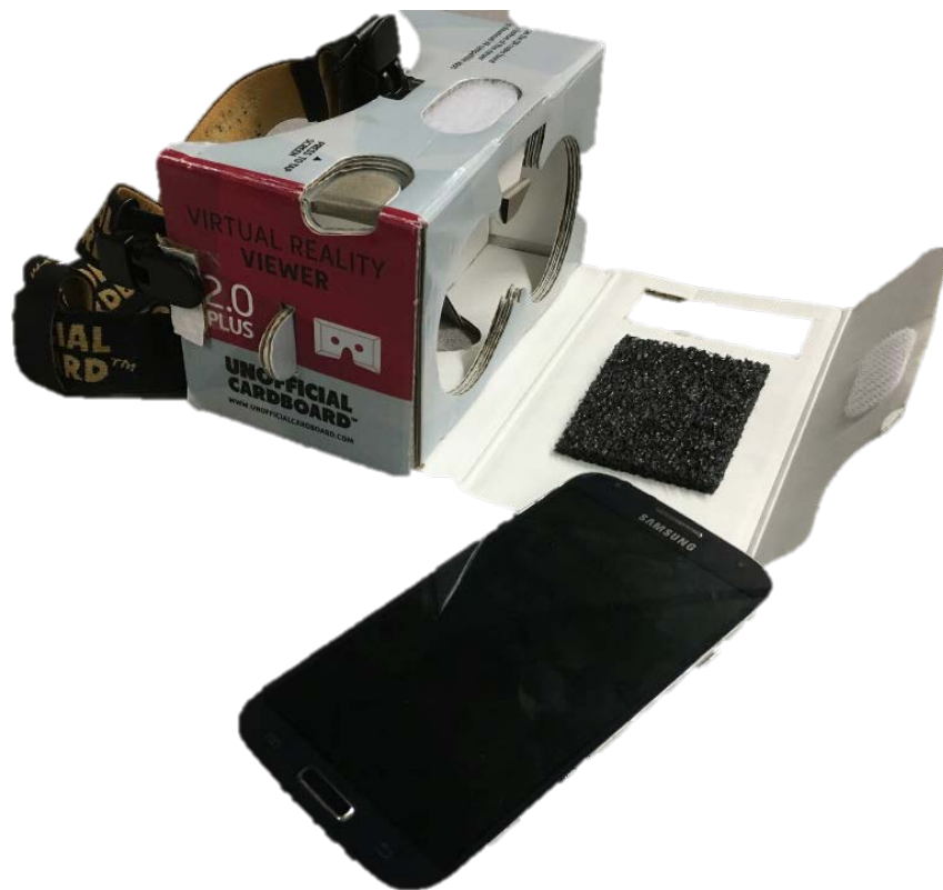
Figure 3.3 MyEyes is made with cardboard goggles and smartphone
