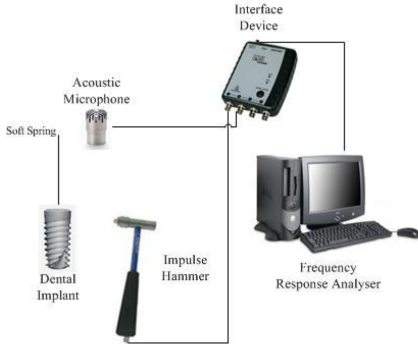
Figure 2-4: Test setup of implant modal analysis
