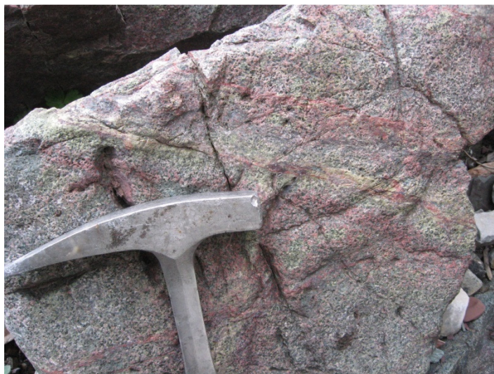
Fig. 6: Medium-grained dioritic Bonnet Plume River Intrusion showing pervasive chlorite alteration and fracture-controlled potassic (red) and epidote (yellowish green) alteration, near the Pika mineral occurrence (Fig. 1, Fig. 11A).
