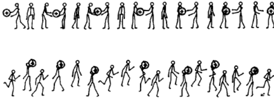
Figure 1.8 Models of proton conduction. Top: Grotthuss Mechanism: protons are passed along the hydrogen bonds. Bottom: Vehicle Mechanism: protons are transported by H 2 O.
