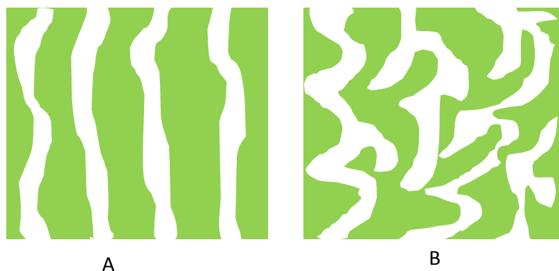
Figure 1.10 Schematically diagram of proton conduction pathway in PEM (white = aqueous domains) where the degree of tortuosity of proton conduction pathway is greater in B than in A
