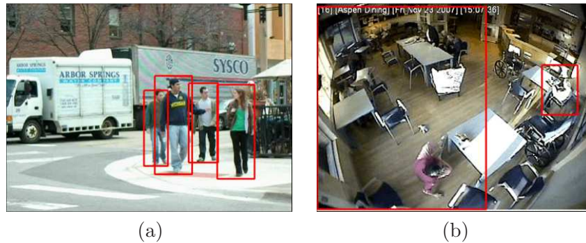
Figure 3.6: Typical results of running a state-of-the-art pedestrian detector [12] on the two datasets used in the experiments. On the collective activity dataset (a), the detector performs very well. But on the more challenging nursing home dataset (b), the detector is not reliable since the videos are captured by a fish eye camera, so persons in the videos are not in upright positions. In addition, the video quality is very poor.
