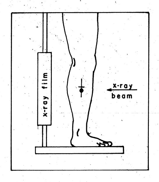
It was necessary to mark the skinfold so that the experimenter could tell where to measure the fat thickness on the radiograph. This was done by taping an English penny to the surface of the skin, 1/2 cm below the skinfold mark. The penny had the added advantage that it could be used as the magnification correction factor measure, since the penny was exactly 2 cm in diameter, and when viewed from the edge was 2 cm from any angle.
